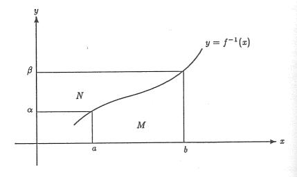
The figure gives a graphical interpretation of (2) in the case where f is increasing. The definite integrals give the areas M and N and the term  $[xf^{-1}(x)]_a^b$  expresses M+N as the difference of two rectangles. A difference picture is needed for decreasing functions — the details are left to the reader.
